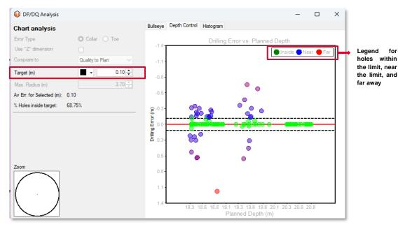
Figure 267 - DP/DQ Analysis - Depth Control Graph.
