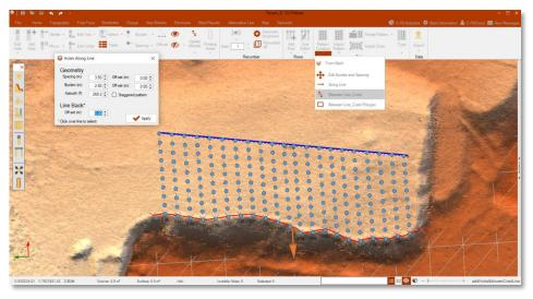
Figure 246 - Pattern creation using between Line\_crest.
