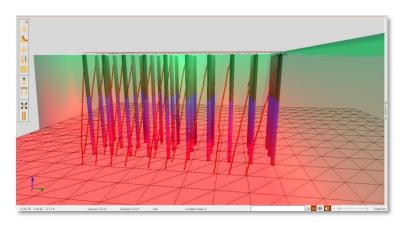
Figure 166 - Borehole deviation information successfully imported.
