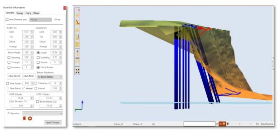
Figure 178 - Changing holes' inclination (no bottom correction).
