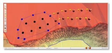
Figure 298 - Selecting detonators.
