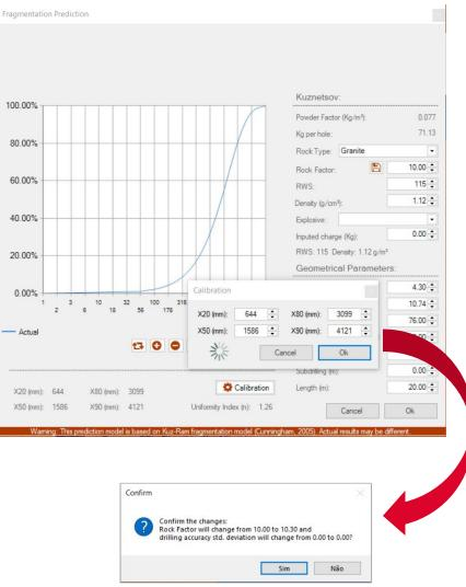
Figure 370 - Calibration of fragmentation and confirmation of rock factor changes.
