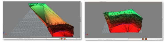
Figure 151 - Outliers detection algorithm results (Left: without outlier detection; Right: With outlier detection).
