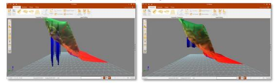
Figure 153 - Borehole length definition (Left: Bench bottom position; Right: Borehole length).
