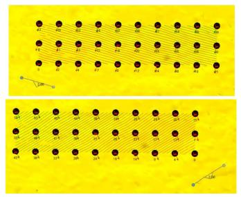
Figure 320 - Two example of blast direction, depending on the polyline position.
