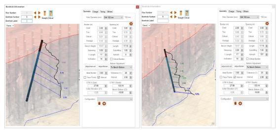
Figure 180 - Adjusting azimuth. A (left): azimuth not adjusted; B (right): azimuth adjusted automatically.
