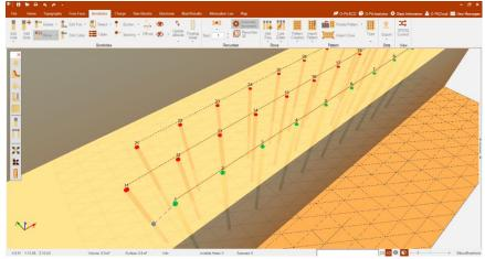
Figure 181 - Moving a single hole.
