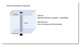
Figure 71 - Volume calculation "By holes".
