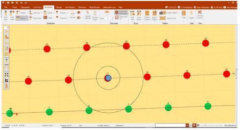
Figure 186 - Move hole using proximity ring.
