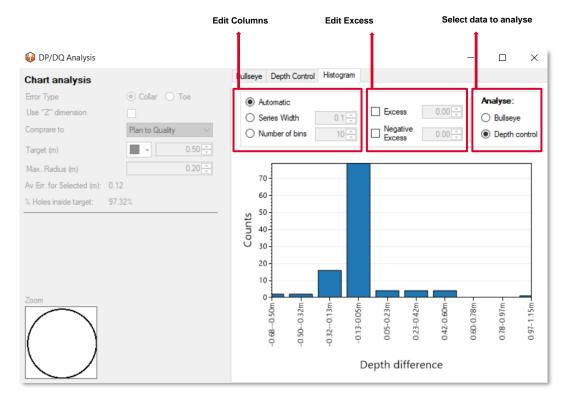
Figure 270 - DP/DQ Analysis - Histogram Graph: Analyse by Depth Control.
