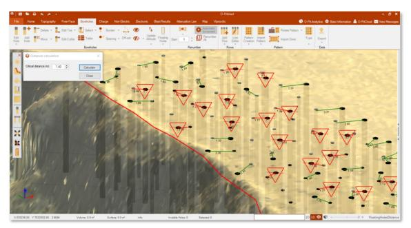
Figure 216 - Critical distance between previous hole (from previous blast) and new hole (for the new blast).
