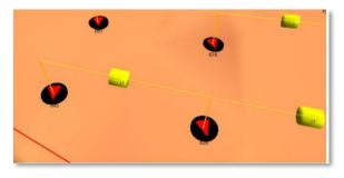
Figure 300 - Surface delays and in-hole detonator visual feedback.
