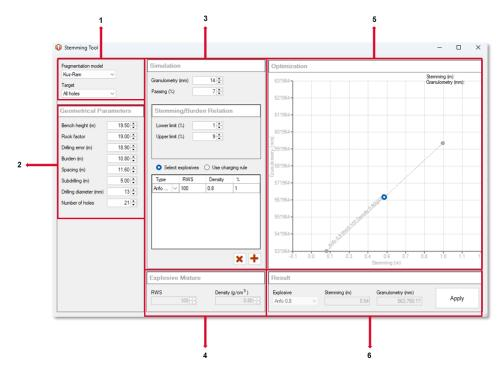
Figure 398 - Stemming Tool window. 1: Fragmentation Model and Target; 2: Geometrical Parameters; 3: Simulation; 4: Explosive Mixture info; 5: Optimization graphic; 6: Result.
