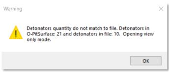
Figure 361 - Warning message when detonators quantity does not match to file.
