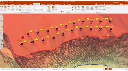
Figure 290 - Non-Electric connections.
