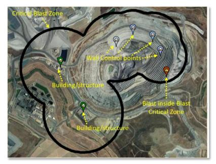
Figure 433 - Critical Blast area.
