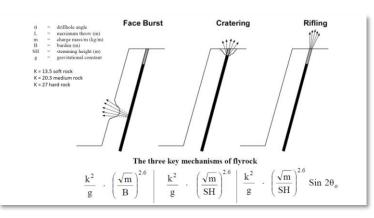
Figure 77 - Face burst, cratering and rifling calculation.
