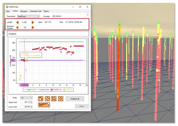
Figure 443 - MWD Data - Outliers Tab: Inspecting Borehole 101 at s 1.435m depth.
