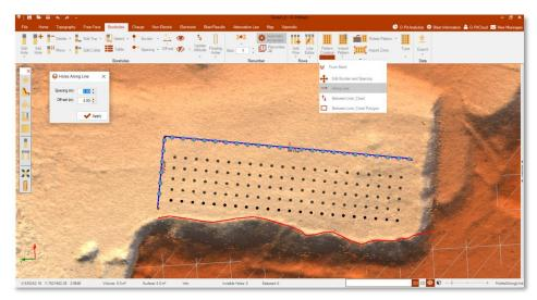
Figure 245 - Pattern creation using along line.
