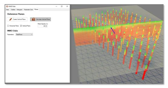
Figure 451 - MWD Data - Planes Tab: Calculating Vertical Plane.
