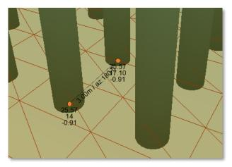
Figure 99 - Distance between two bottoms (CRTL + click on orange spheres).
