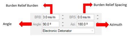
Figure 317 - Parameters that change the direction vector.
