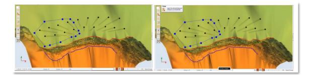
Figure 282 - Applying charge rule to a selection of holes.
