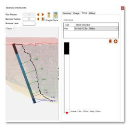
Figure 293 - Editing In-Hole detonator.
