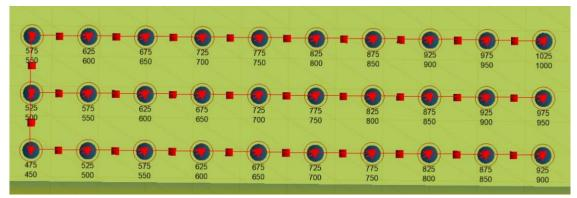
Figure 308 - One deck per hole (decks with connector of 450ms).
