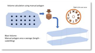
Figure 75 - Volume calculation using manual polygon.
