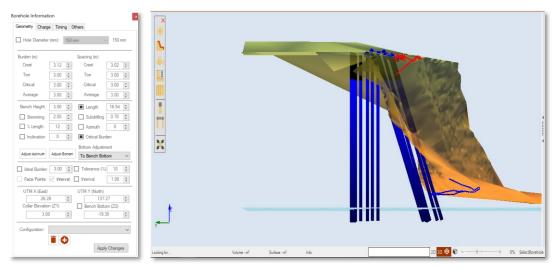
Figure 179 - Changing holes' inclination (with bottom correction).
