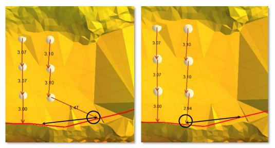
Figure 203 - On the left: first position of the burden; on the right: new burden position.
