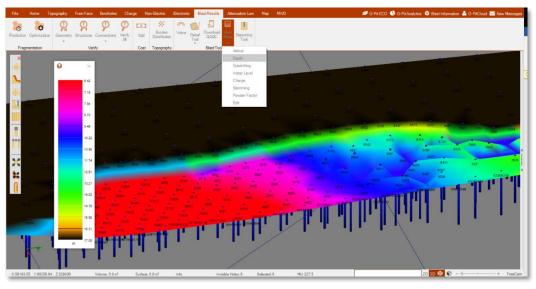
Figure 396 - Heat Map tool example showing variations in depth.
