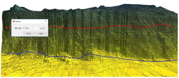
Figure 162 - Example of changed altitude in crest (minus 5 meters from top).
