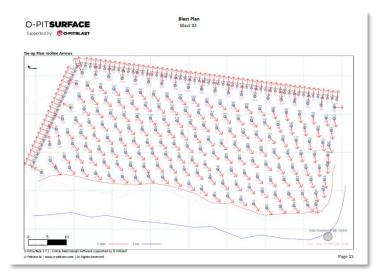
Figure 47 - Tie-Up Plan: Isoline Arrows.
