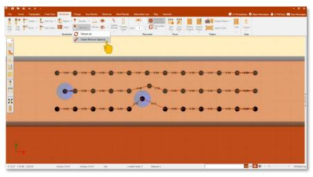
Figure 206 - Check minimum spacing tool.
