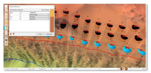
Figure 283 - Applying different charge rule using length as parameter.
