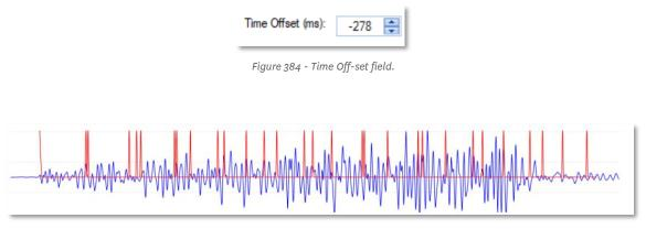
Figure 385 - Seismographic information combined with the detonation time of holes.
