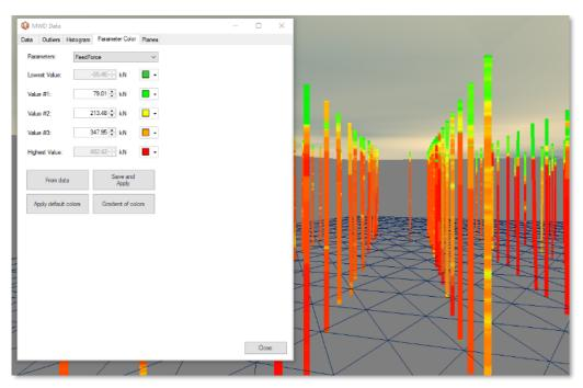
Figure 447 - MWD Data - Parameter Color Tab.
