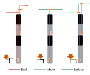
Figure 307 - Type of deck connections.
