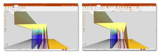
Figure 210 - Left (a): visible boreholes; Right (B): invisible boreholes (with deviation data).
