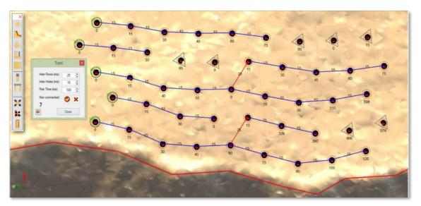
Figure 325 - Timing between Rows and holes.
