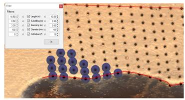
Figure 379 - Filter Holes by Geometry window.
