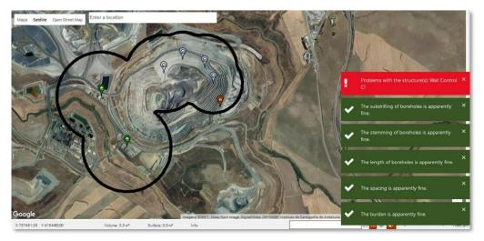
Figure 434 - Detection of problems with the structures.
