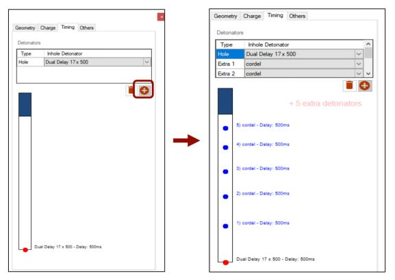
Figure 315 - Adding extra detonators.
