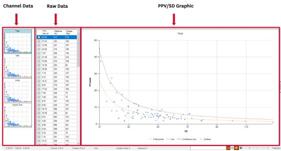
Figure 403 - A: Channel data; B: Raw data; C: PPV/SD Graphic.
