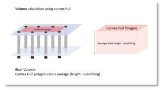
Figure 73 - Volume calculation using "Convex Hull".
