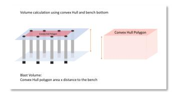
Figure 74 - Volume calculation using convex Hull until bench bottom (instead of holes average length).
