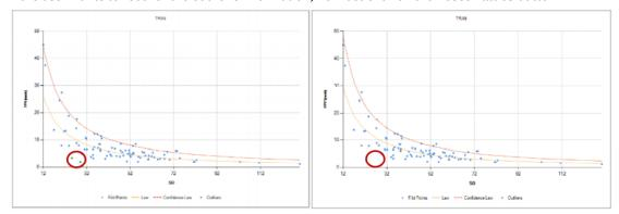
Figure 408 - Left (A): PPV/SD Graphic with outliers; Right (B): PPV/SD Graphic without outliers.
