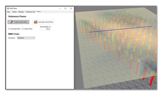
Figure 450 - MWD Data - Planes Tab: Creating Vertical Plane
