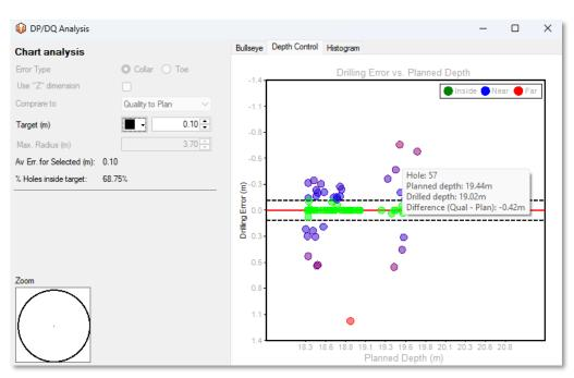
Figure 268 - DP/DQ Analysis - Depth Control Graph - Information displayed on mouse hover.
